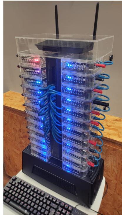
Fig. 1. UP Cluster at Insper. shows the operational Up cluster in the networking and HPC laboratory. Documentation available at <https://insper.github.io/UpCluster/>
