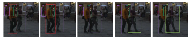
Figure 9. Example of an ID theft case. Note that between the second and fourth image, the object with id=2 loses it and receives the ID of the object next to it as a new value.
