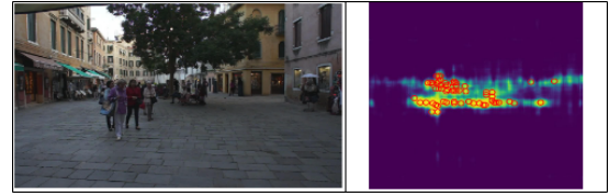
Figure 5. Example of an image with heatmap detection and its peaks. A concentration of people is noticeable in the central region, with empty areas in the upper and lower regions, demonstrating good model capability.
