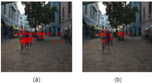
Figure 7. Image (a) shows the detections over the image before applying NMS step. Image (b) shows how the detections become after applying NMS.
