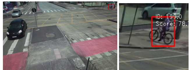
Figure 11. Unaccounted cyclist. In the left image, the cyclist appears at the upper right corner, identified by the red bounding box. This area has been enlarged in the image on the right.
