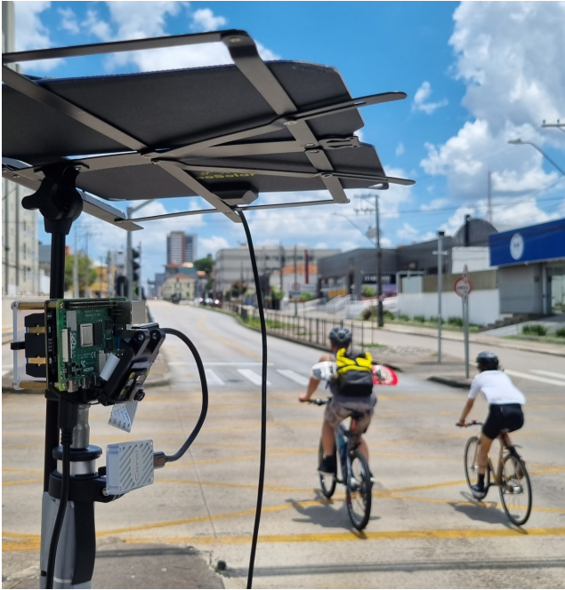
(a) All devices connected and the camera tilted at an angle of approximately 25^\circ .
