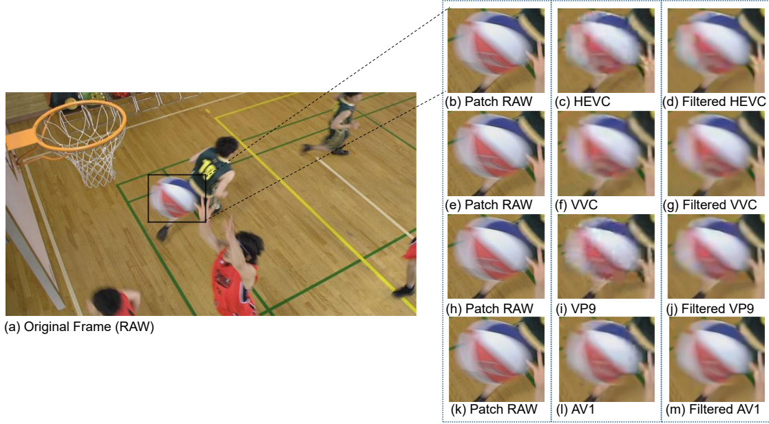
Figure 7. Frame number 14 of the BasketballDrill sequence: (a) Original frame (RAW); (b)(e)(h)(k) Cropped section of the original frame; (c) HEVC-decoded version; (d) Enhanced HEVC-decoded version; (f) VVC-decoded version; (g) Enhanced VVC-decoded version; (i) VP9-decoded version; (j) Enhanced VP9-decoded version; (l) AV1-decoded version; (m) Enhanced AV1-decoded version.
