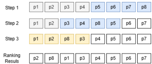
Figure 3. Sliding Window Strategy. An example demonstrating the re-ranking of eight passages using a sliding window approach with a window size of four and a step size of two. The blue-colored segments indicate the first two windows, while the yellow segment represents the final window. The sliding windows are applied in a back-to-first sequence, ensuring that the first two passages from the preceding window contribute to the re-ranking process in the subsequent window. [Sun et al. , 2023]
