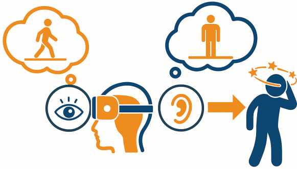
Figure 7. In this illustration, a person is using a head-mounted display (HMD) to view immersive content while standing. This creates a conflict because, although the eyes perceive movement through the HMD's screen, the vestibular organs in the inner ear are sending signals to the brain indicating that the person is stationary. This sensory conflict can lead to symptoms of cybersickness.
