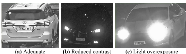
Figure 3. Examples of infrared images under varying conditions: (a) optimal visibility with enhanced perception, (b) reduced contrast affecting detail clarity, and (c) overexposure caused by vehicle headlights.
