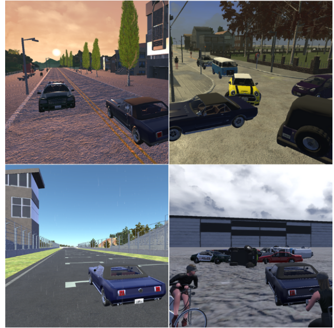
Figure 3. CARLA simulator environments: four different urban maps under varied weather and lighting conditions, demonstrating the simulator’s capability for diverse scenario generation [Dosovitskiy et al. , 2017]. Our experiments used the Town01 map under Clear Noon, Hard Rain Sunset, and Hard Rain Noon conditions.
