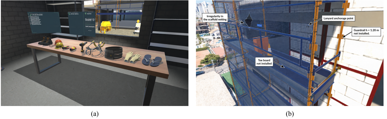
Figure 4. The two zones of the implemented scenario. (a) The Group 1 PPE workbench, holding the five required items and the distractors (helmet without chin strap, abdominal belt, latex gloves, and open-toe footwear). (b) The Group 2 scaffolding platform, with the four seeded irregularities annotated: missing guardrail, missing toeboard, disconnected lanyard, and fallen safety net.
