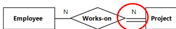
Fig. 5. Example of advanced structural constraint on an N:N relationship with total participation on either side
