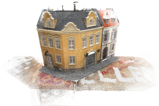
Figure 11. Ground truth point cloud of the set6 from the DTU MVS dataset.
