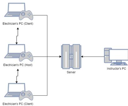
Figure 1. Overall architecture of the project.
