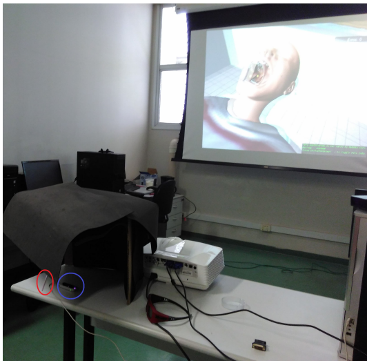
Figure 4. Environment with the use of a straw (red circle) that represents a virtual syringe and Leap Motion (blue circle) for virtual tool tracking. In order to prevent interference caused by the infrared rays emitted by the Leap Motion device on the shutter glasses, a specially designed apparatus made of cardboard and ethyl vinyl acetate (EVA) sheets was used.
