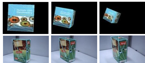
Figure 18. IPB tracking results for a synthetic sequence (top) and a real sequence (bottom).
