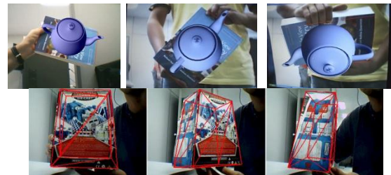
Figure 22. KB results using SIFT and LM with planar (top) and non-planar (bottom) objects.
