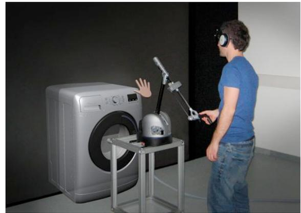
Figure 4. Multimodal interaction with the Virtual Prototype of a washing machine
