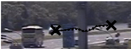
Fig. 6. Example of a tracked vehicle using the proposed adaptive particle filtering approach. The crosses indicate the initial and final tracked vehicle positions, and the dotted line the tracked vehicle path. The solid line shows the vehicle path interpolated to reduce the occlusion edge effect.
