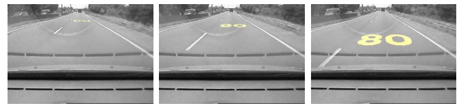
Fig. 8. Frames illustrating the automatic camera calibration procedure, and the insertion of a virtual horizontal sign.
