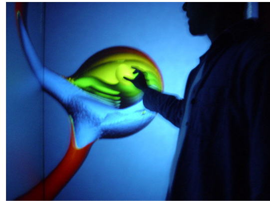
Figure 9. CAVE displaying blood vessels with flow speed in colours.
