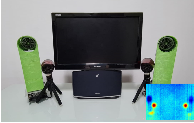
Figure 1. The TWIRL prototype consists of two pairs of cold (green) and hot wind (red) devices that can work with both a screen and a VR headset. The bottom right corner features a thermal image illustrating the devices in an operational state. Red means heat, whereas dark blue is coldness [Rodrigues et al. , 2021].
