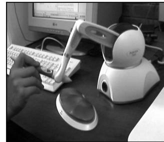
Figure 1. Phantom Omni haptic device used in VR systems and in the Bone Marrow Harvest simulator.
