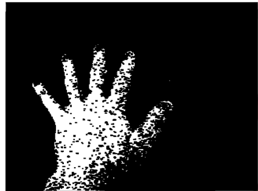
(b) The result of erosion on the image 7a.
