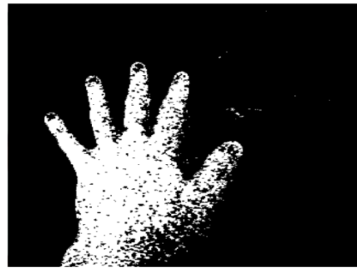
(a) Noisy binary image resulting from colour range segmentation for the skin on the H channel.
