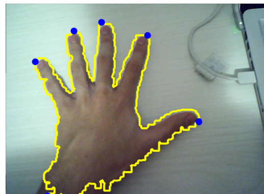
(d) Finger tracking based on the convex hull.
