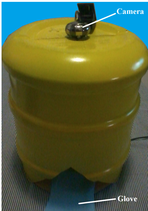
Fig. 5: Materials used to create the controller. The 20 L mineral water bottle was painted so it could block any outside incoming light.
