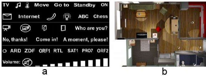
Fig. 8. A (a) P300-based BCI for controlling (b) a virtual domotics environment. Source: [44].
