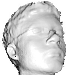
Fig. 3. An example of user's head reconstructed with the KinectFusion and rendered with Phong shading [22].
