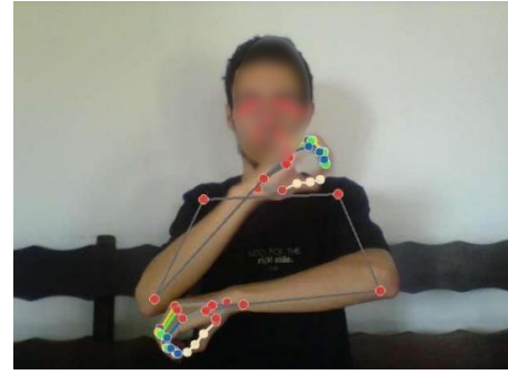
Figure 6. Mediapipe Pose and Hands printed in comparison over a frame
