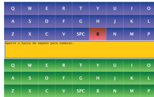
Fig. 1. Virtual keyboard for eye typing based in the context switching paradigm, image reproduced from [15]
