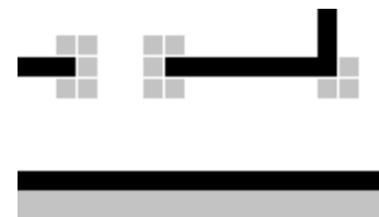
Fig. 11. Regions to avoid during planning are marked in gray and walls in black.
