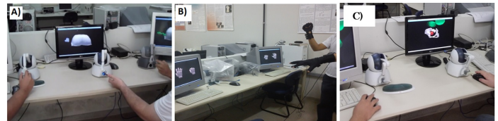
Fig. 5: Tutoring CVE with bidirectional tele-haptics, developed with CyberMed . The user at left controls the movements of other remote users.
