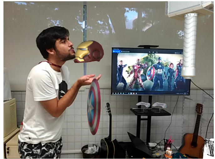
Figure 19. Picture taken by user with bad tracking result. It is possible to notice that the tracking is not accurate just by comparing the 3D position of the virtual objects relative to the TV.
