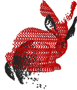
Fig. 9: Best registration (ICP CTFSF, with k = 75\% ) obtained for the 90^\circ - 180^\circ case. All the registration methods of Section III get incorrect results in this case.
