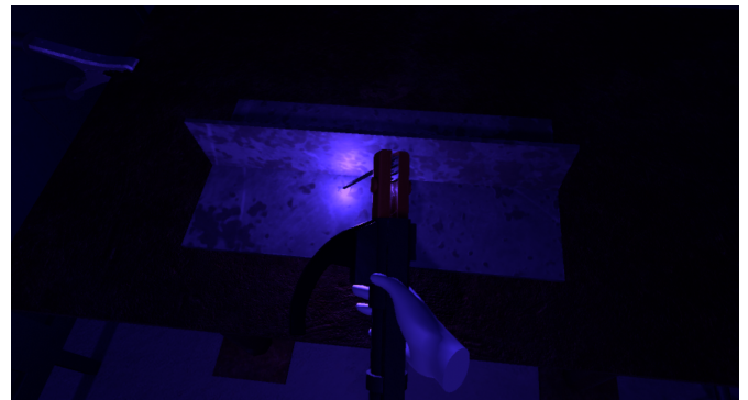
Figure 7. Welding process with visual effects. The mask automatically darkens when the arc ignites, simulating the activation of the welding helmet filter.
