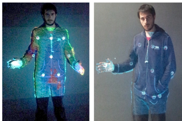
Figure 16 - Left: Depth Mapping with a Cyclic Scale. Right: Depth Mapping with a Two Color Scale. In both cases the skeleton mapping overlaps the corresponding mapping.
