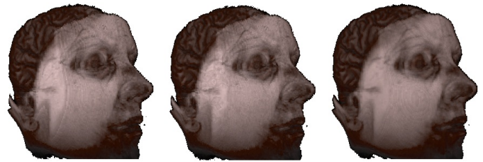
Fig. 8. A volume rendering (left) with stochastic jittering (center) and tri-cubic filtering (right). The stochastic jittering reduces the wood-grain artifacts in the volume, however it is almost imperceptible in this scene. The tri-cubic filtering smoothes the volume data, reducing the artifacts present in the volume rendered with trilinear filtering.
