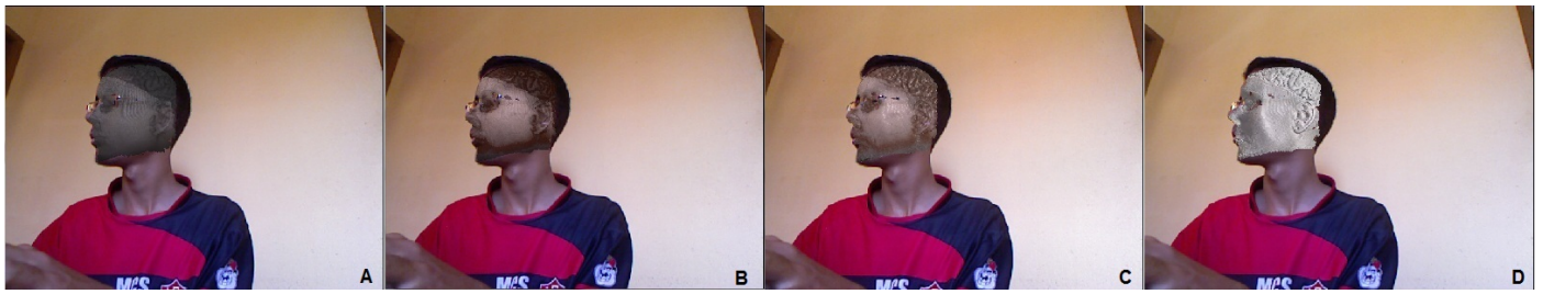
Fig. 3. Some of the visualization options. A) Direct volume rendering (DVR). B) DVR with pre-integrated transfer function. C) DVR with pre-integrated transfer function and Blinn-Phong illumination. D) Non polygonal iso surface volume rendering.
