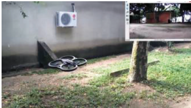
Fig. 24. Open field navigation test. Screen on top right shows image viewed on Glass and captured by AR.Drone's camera.
