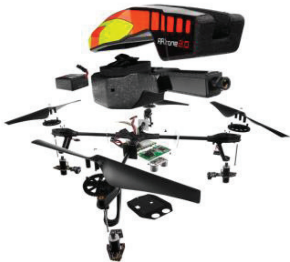
Fig. 18. AR.Drone 2.0 components ( http://ardrone2.parrot.com/ ).
