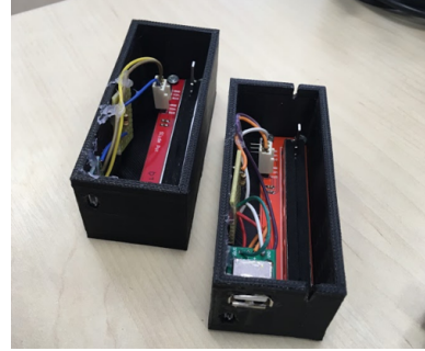
Figure 3. Linear potentiometers used to measure braking intensity.
