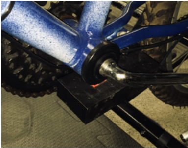
Figure 2. Mouse positioned to capture the axle's protection cover rotation.
