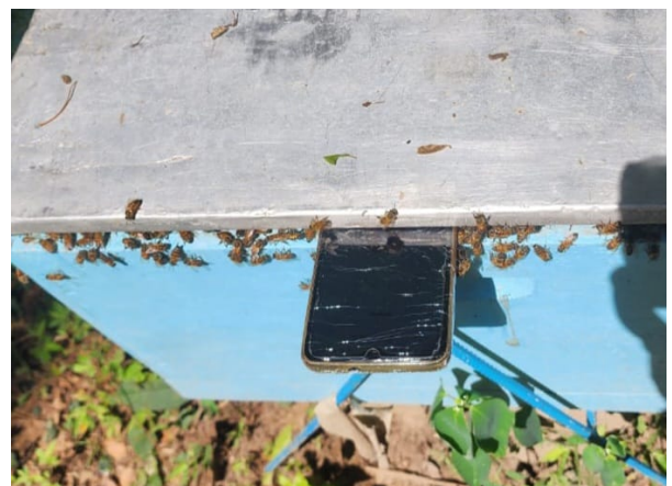
Figure 2. Hive audio acquisition in a real-world apiary setting. Audio is recorded by placing a smartphone with its microphone facing inside the hive, positioned between the lid and the box. The smartphone is wrapped in plastic film to prevent bees from covering the device with propolis.
