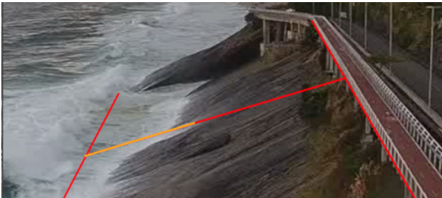
Figure 3. Example of lines used to compute the wave height based on the defined curves. The orange line represents the fitted segment, while the red line represents auxiliary lines.
