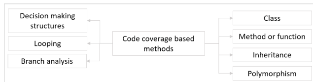
Figure 7. Main aspects used in source code coverage-based methods.
