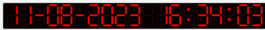
Figure 13: LLCTT Date/Time Display. Local Time Is Stored In The CMOS Battery And Can Be Changed In The BIOS, In The Operating System, And Through The LLCTT.
