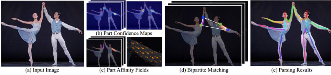
**Figure 1. Pipeline of the OpenPose method [Cao et al. 2018].**
