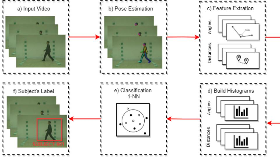
**Figure 4. Block diagram of the proposed method for gait recognition using 2D poses.**
