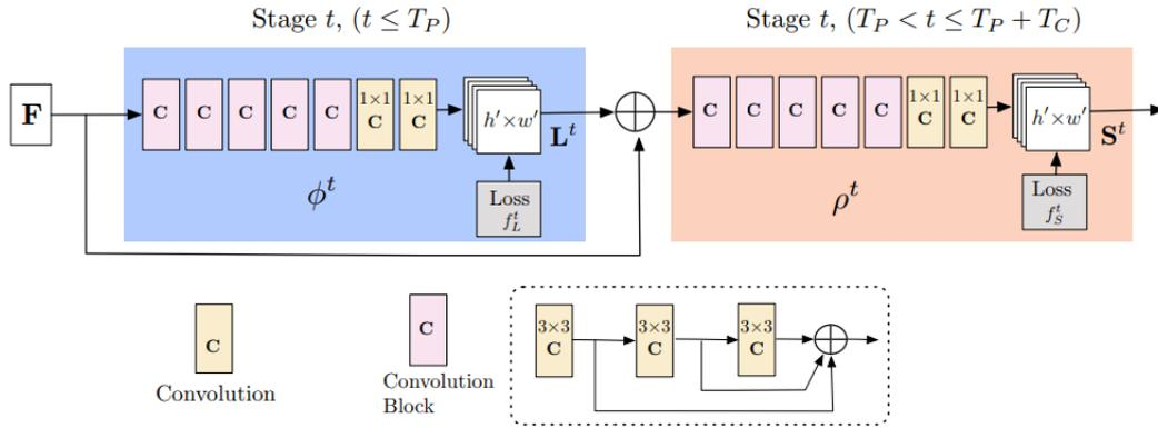
**Figure 2. OpenPose CNN architecture [Cao et al. 2018].**
