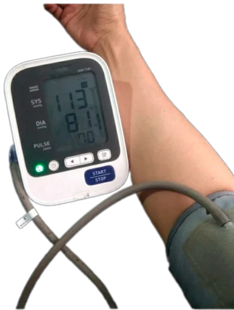
Figure 2. Digital and automatic blood pressure measuring device. Oscillometric method. Adapted from: Hsu et al. [2020]
